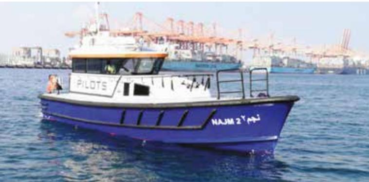
The pilot boats have been given the series name of Najm, which means “star” in Arabic drawing inspiration from the traditional use of stars for vessel navigation. Najm-2 is manufactured by Damen Shipyard in Antalya, Turkey. It’s a high speed vessel with state-of-the-art navigation systems fitted and special propeller tunnels to increase propulsion efficiency, reduce draft, vibration
